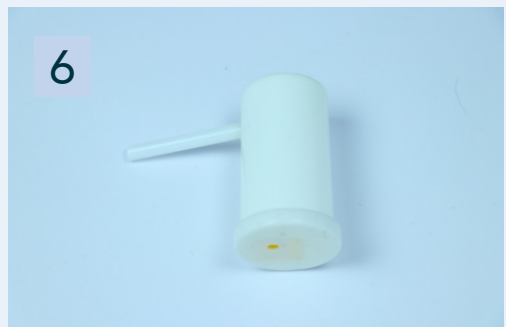
Insert a stiff straw in the side hole. Apply some glue to make the connection airtight.
