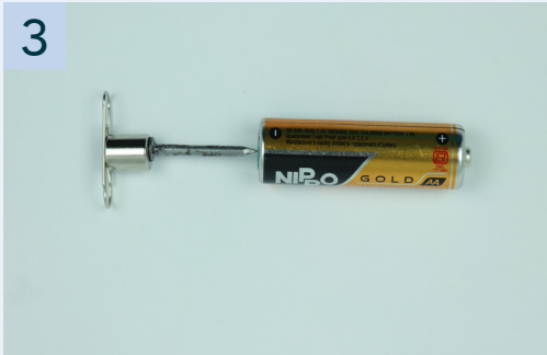
3 Add the screw on the negative terminal of the battery.
