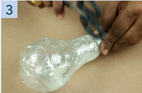
Break the glass from the bottom to detach it from the bulb.
