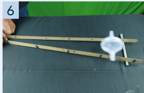
6 Surprisingly, you will find this roller climbs from the lower end of to the higher end on its own.
