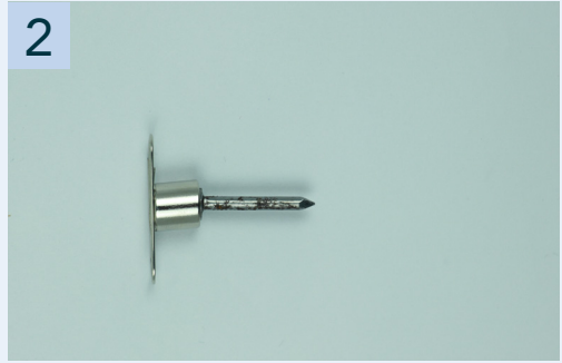
2 Place the neodymium magnet on the head of the screw.
